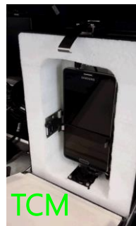
TCM "Terminal Container Module": (+) the UE uses the built in RF antennas
