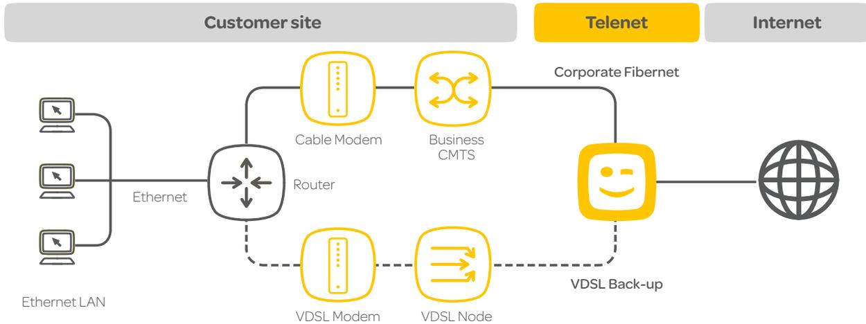
Figure : Configuration technique Corporate Fibernet
