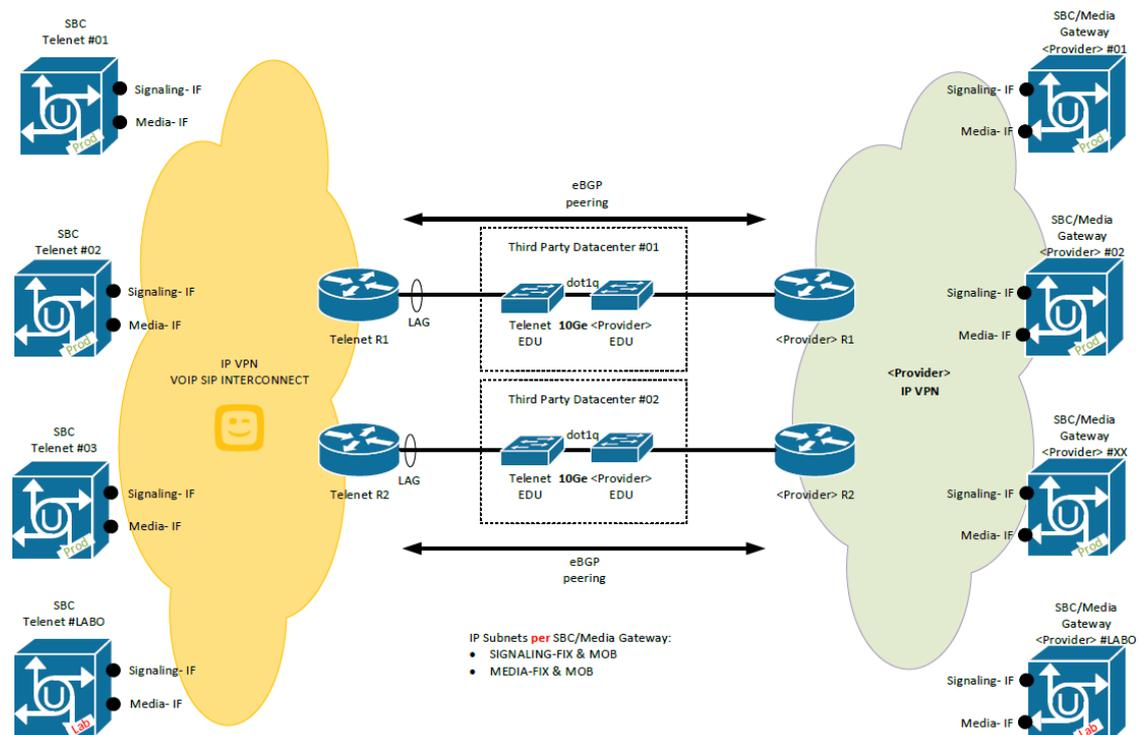
The demarcation point between the two networks is the patching between the two EDUs. The Party having ordered the patching to data centre is liable for the patching itself.
